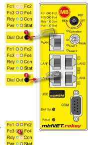
If the flashing frequency of the LED Con is 3 Hz, the device is attempting to log into the portal. If the login has been successful, the flashing frequency is reduced to 1.5 Hz.
